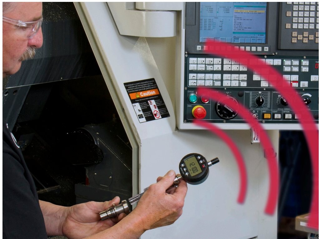
▲ A fixed plug comparative gage allow the operator to get the best measurement with no operator influence.
