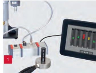
1 Pneumatic module in use with a nozzle ring gage
