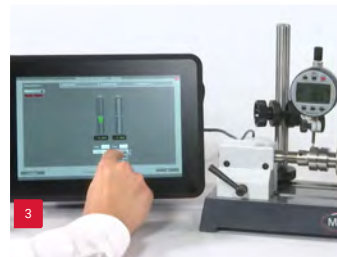
3 Radial run out measurement with dial indicator
