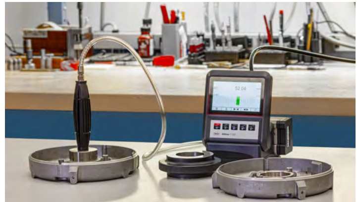
Stand alone air gaging for bore diameter
