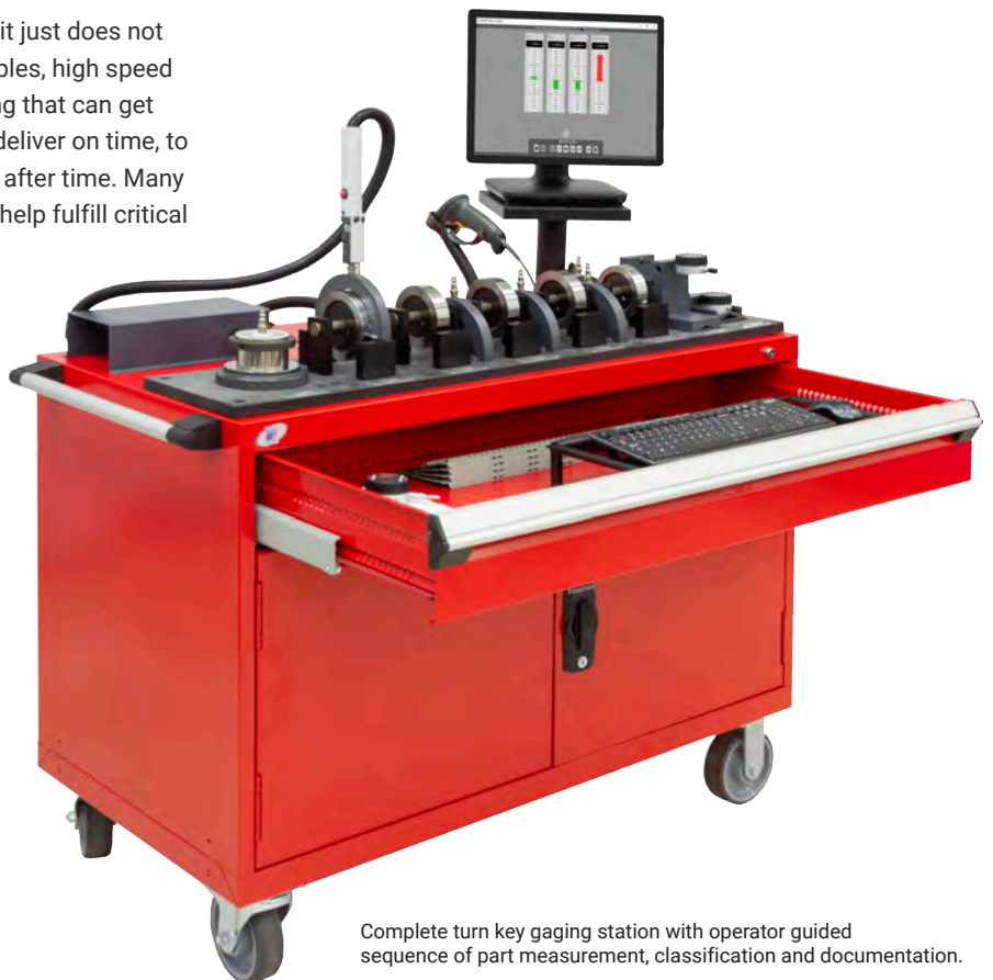
Stand alone air gaging for bore diameter
