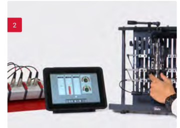
2 Shaft measurement with inductive modules
